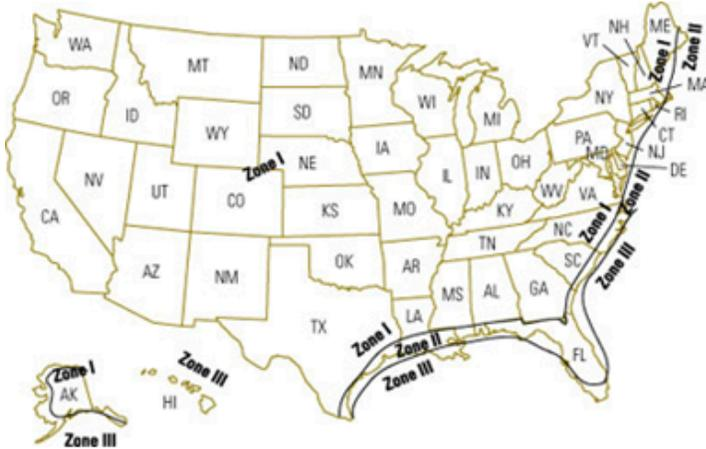
Wind zones were created by HUD with the 1976 changes. These wind zones are designed for horizontal wind speeds and uplift loads.
